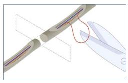
2. The selected fibre unit (ESFU) can be extracted and cut. This operation is performed some floors above the floor where the customer is to be connected.
