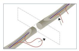
3. At the floor where the fibre connection is requested, the ESFU that was cut on the higher floor can now be easily extracted.
