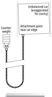
There are a couple of methods in use to counterbalance long lengths of compensation. Some companies actually supply static weights that hang from the car opposite the compensation attachment point. While this does counterbalance the compensation, it lowers the capacity and overall performance of the car by making it heavier.
