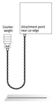
Compensation forms a loop as it hangs from its attachment points. The width of that loop depends on the flexibility of the compensation. Like the materials it replaced, compensating cable forms a fairly narrow natural loop. Note that the compensation is attached near the edge of the car because of this narrow loop.
